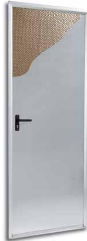
The inner nucleus comprises a bee's nest network in 18mm alveolar structure which gives a resistance to compression of 1.2kg per cm<sup>2</sup>. The adhesive used is applied using the hot gluing process and then pressed to achieve a traction resistance value of 0.32 kg per cm<sup>2</sup>.
